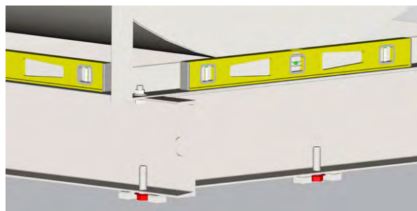
Carefully level the fan on the foundation
