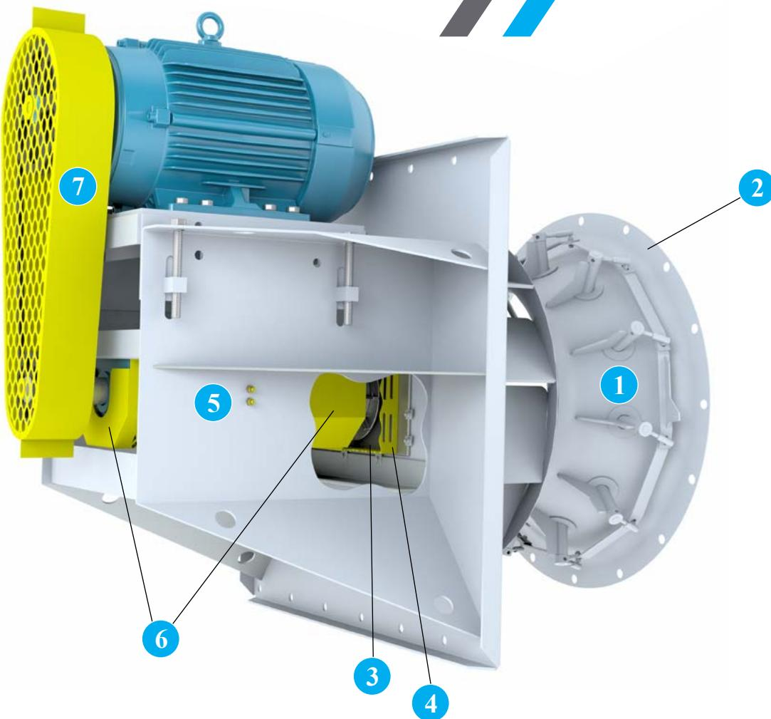
**1 Variable Nested Inlet Vanes** Vane blades are cantilever design or center supported, equipped with permanently lubricated bearings and ball joints for smooth and easy operation. See page 5 for more information.
