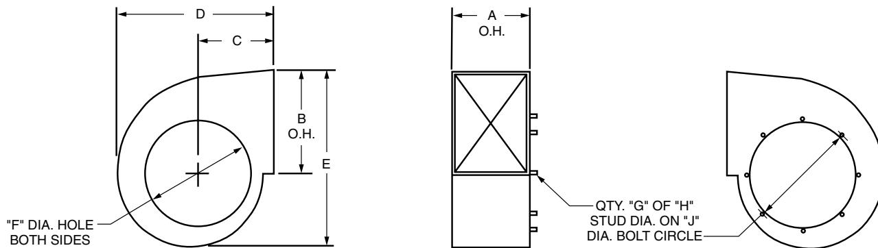
NOTE: Rotation must be specified as viewed from drive side to ensure proper location of inlet cone mounting studs.
