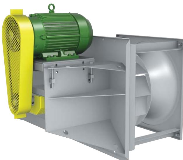
Plug fans offer great versatility for complex system configurations. Equipped with a gusseted mounting panel, they are mounted directly to the plenum wall separating the motor and drive components from the process air. Plug fans provide high efficiency recirculation air with the benefit of easy installation and removal.
